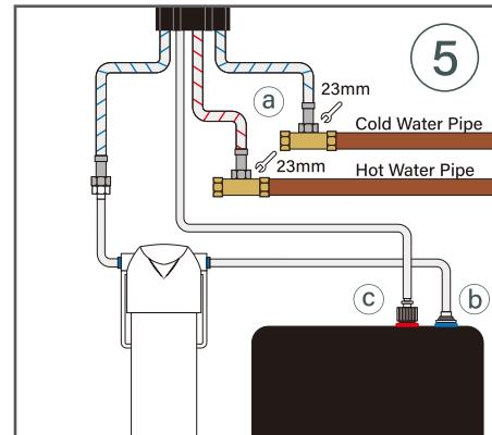
5(b). Connect hose for cold water from tap to boiler.
